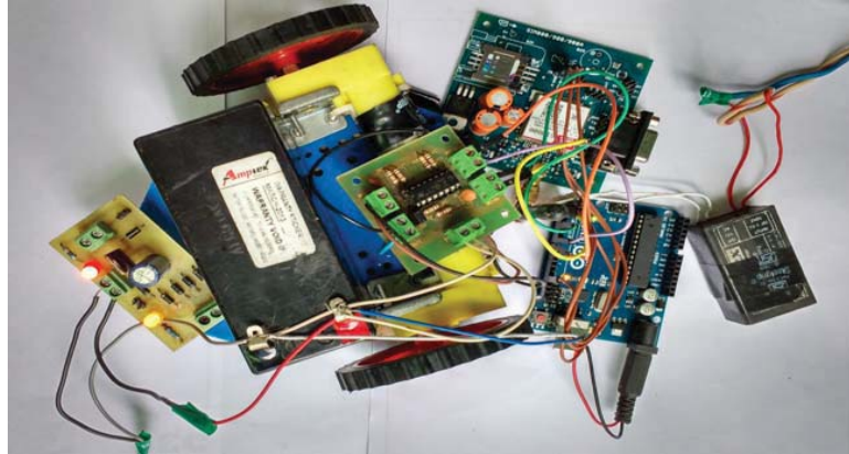
Fig. 8 GSM controlled robot through wireless power transfer
