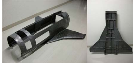
Fig. 14 Full composite semi-monocoque structure of WIRES#014
