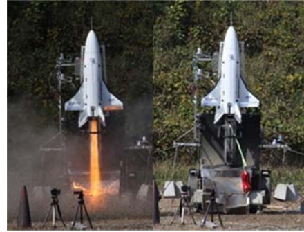
Fig. 17 Third ground combustion test of WIRES#014
