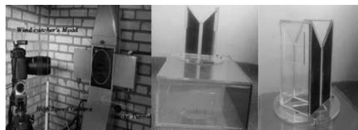
Fig. 8 Experimental setup and wind-catcher model
