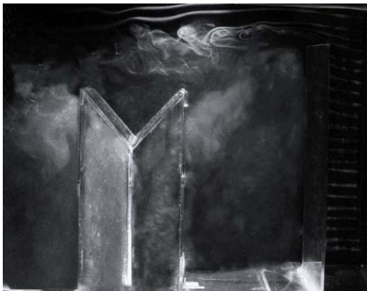
Fig. 13 Visualized flow pattern around and inside the two-sided wind-catcher with upstream structure ( h=1.25H & X=0.75H )
