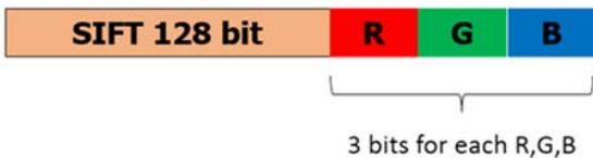
Fig. 6 Moment color-SIFT descriptor with 9-bit RGB format
