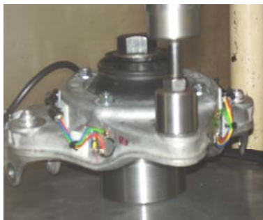
Fig. 8 Physical test to measure strains
