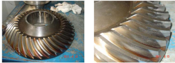
Fig. 19 Bevel gear engaged with pinion
