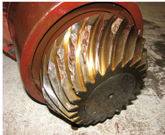
Fig. 16 Damaged gear (pinion)
