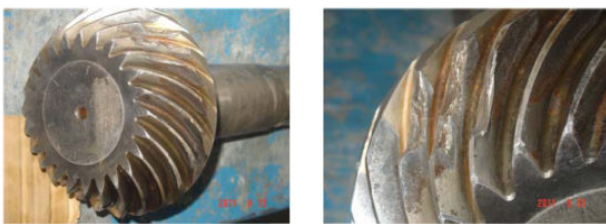
Fig. 18 Damage in gears in the next stage
