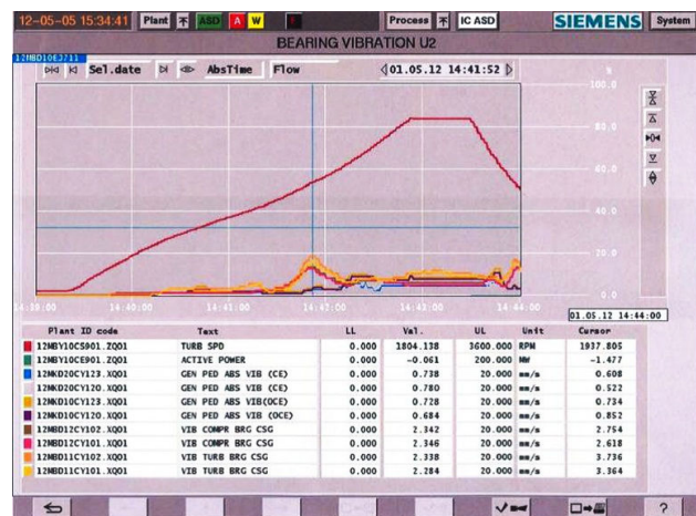
Fig. 15 Typical board monitoring system
