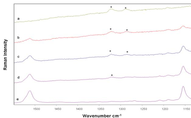
Fig. 3 Raman spectra of beta-carotene in admixture with usnic acid (Asterisks indicate usnic acid bands): (a) usnic acid (b) 0.25mg kg<sup>-1</sup> (c) 0.50mg kg<sup>-1</sup> (d) 1mg kg<sup>-1</sup> (e) 5mg kg<sup>-1</sup>
