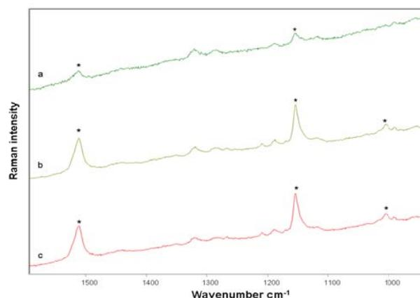
Fig. 2 Raman spectra of beta-carotene in admixture with usnic acid (Asterisks indicate beta-carotene bands): (a) 0.25mg kg<sup>-1</sup> (b) 0.50mg kg<sup>-1</sup> (c) 1mg kg<sup>-1</sup>
