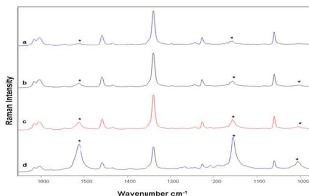
Fig. 5 Raman spectra of beta-carotene in admixture with triphenylene (Asterisks indicate beta-carotene bands) (a) 0.25mg kg<sup>-1</sup> (b) 0.50mg kg<sup>-1</sup> (c) 1mg kg<sup>-1</sup> (d) 5mg kg<sup>-1</sup>
