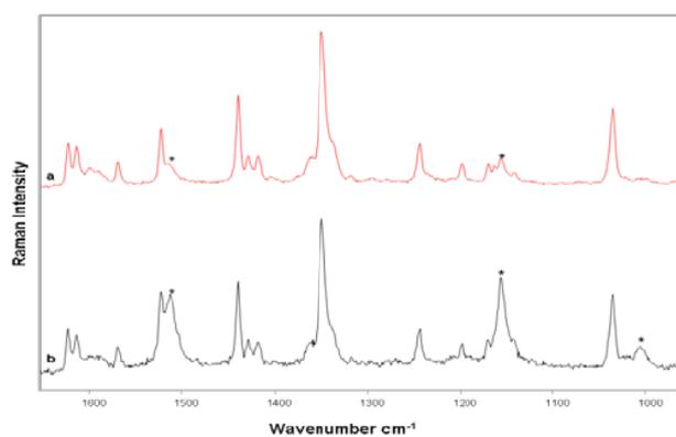
Fig. 4 Raman spectra of beta-carotene with phenanthrene mixture (Asterisks indicate beta-carotene bands): (a) 0.25 mg kg<sup>-1</sup> (b) 0.50mg kg<sup>-1</sup>
