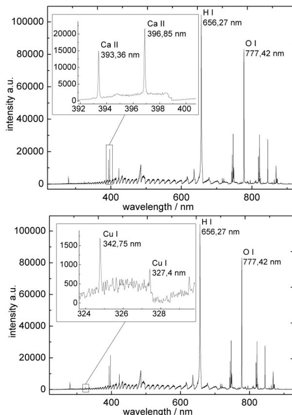
Fig. 3 LIBS spectra of selected elements (calcium, copper)
