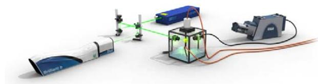
Fig. 1 LIBS system arrangement employing water jet
