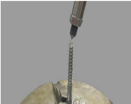
Fig. 4 Spike used for calibration of the rotational table
