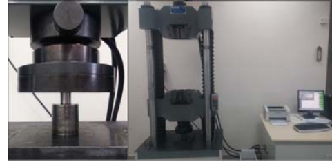
Fig. 4 Hydraulic Press and fixation of parts
