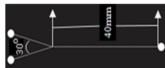
Fig. 2 Structural design of micro-mixer
