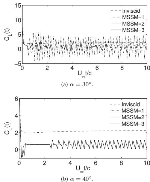
Fig. 12  $C_L(t)$  of a suddenly moving  $NACA4409$  wing,  $AR=9$
