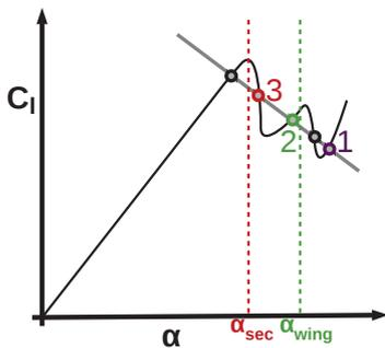
Fig. 6 Multiple Solutions at post-stall angle of attack
