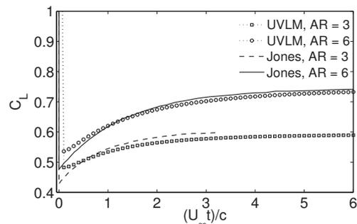
Fig. 7 Transient  $C_L$  of a suddenly moving elliptic wing
