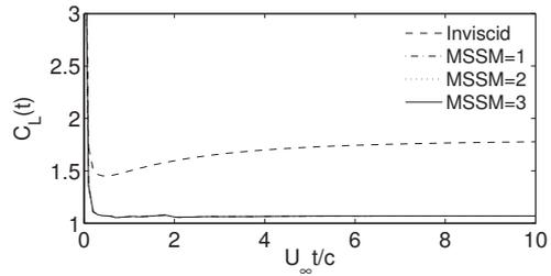
Fig. 11  $C_L(t)$  of a suddenly moving  $NACA4409$  wing,  $AR=9$ ,  $\alpha = 20^\circ$ .
