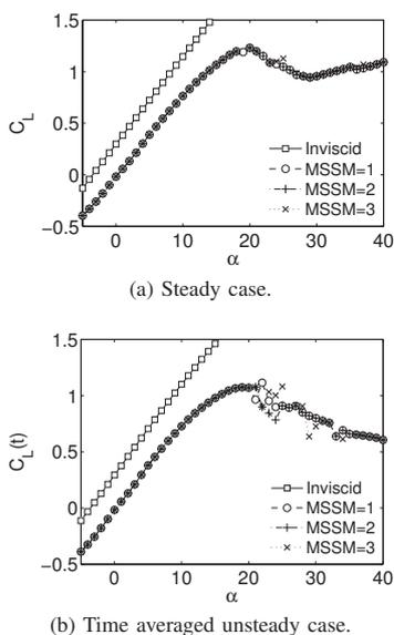
Fig. 10  $C_l$  vs  $\alpha$  for a rectangular  $NACA4409$  wing,  $AR=9$
