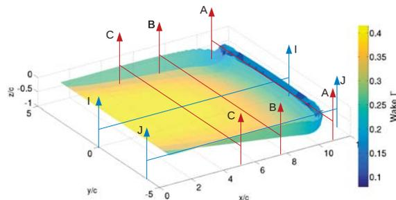
Fig. 16 Wake behind a 3D decambered wing
