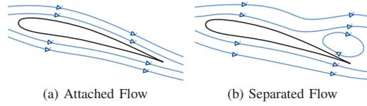
Fig. 3 Flow over an airfoil
