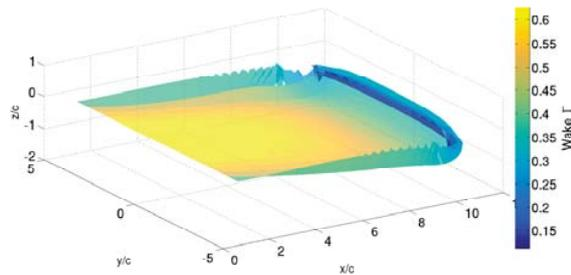
Fig. 15 Wake behind a 3D inviscid wing.
