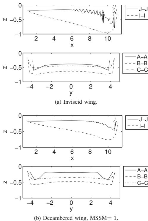
Fig. 17 Cross section of wake at  $t = 10$
