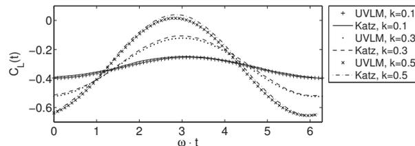
Fig. 8 Transient  $C_L$  of plunging wing
