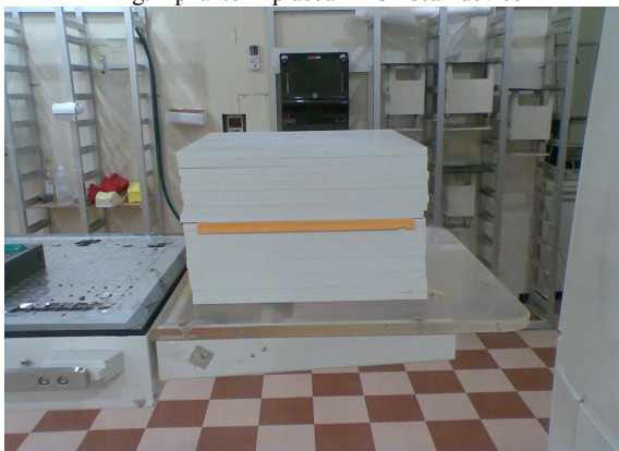
Fig. 2 set up for solid water phantom Plate
