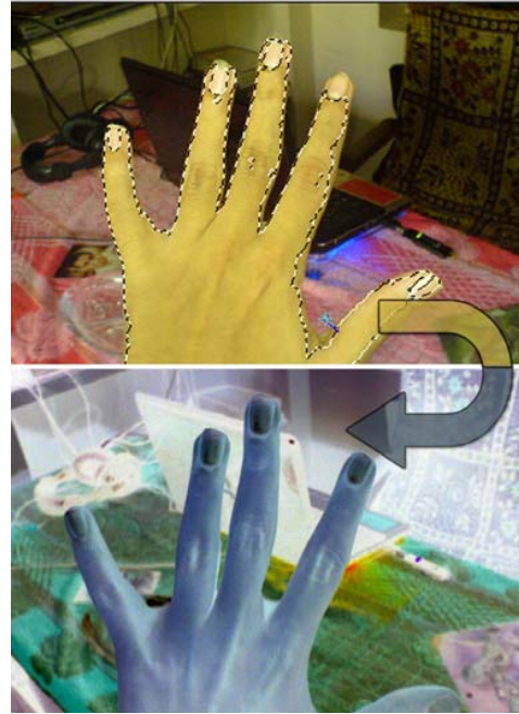
Fig. 5 Color Complexity Reduction through negation
