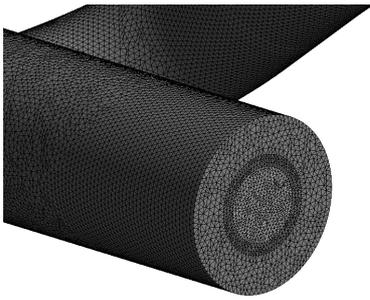
Fig. 6 FEA computational mesh - header
