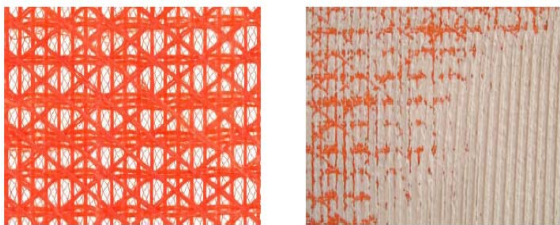
Fig. 2 The hybrid multiaxial seismic textile
