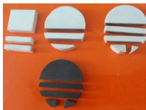
Fig. 6 Corundum ceramic materials with different compositions and experimental specimens fabricated from them
