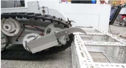
(a) The front end of the vehicle will pass the stair obstacle
