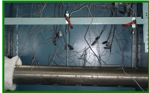
Fig. 9 Photograph of the state of CT before ballooning experiment
