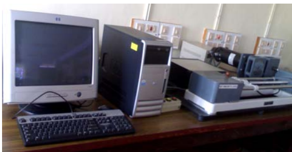
Fig. 4 Electronic Tensometer Apparatus
