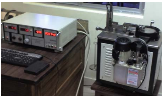
Fig. 5 Wear and Friction Monitor TR – 201CL
