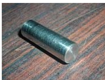
Fig. 2 Wear Test Specimen
