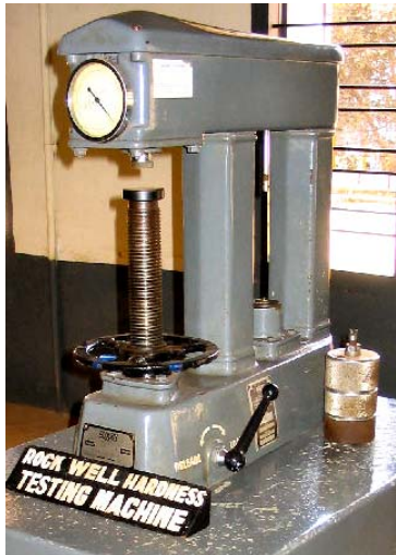
Fig. 6 Rockwell Hardness Testing Machine
