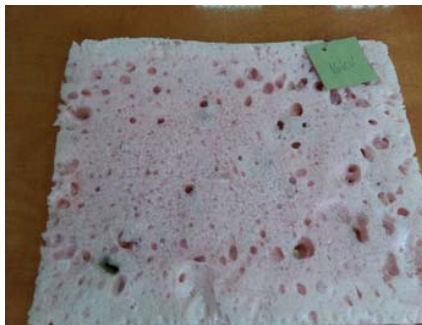
Fig. 4 Fireproof material – expanded polyurethane foam - mastik
