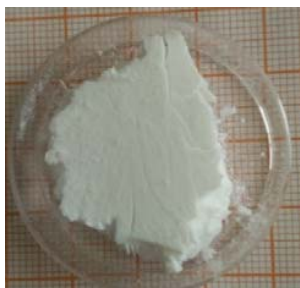
Fig. 4 The sample of aluminum-silicon aerogel
