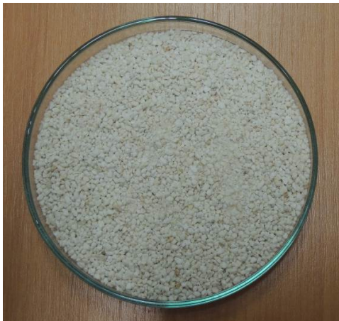
Fig. 1 Demonstration aggregates derived from volcanic glass
