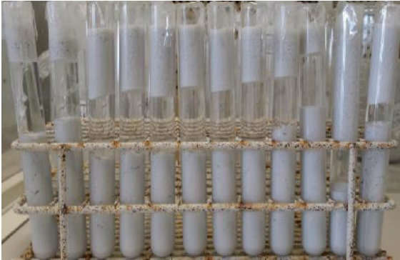
Fig. 8 Samples at different pH values from 4 to 7.5, at 0.1 wt.% SDBS
