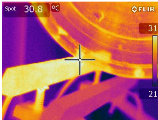
Fig. 14 Thermal spectrum of the sliding contact system for the test current of 8A, contact force of 10N and emissivity coefficient of 0.95
