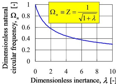
Fig. 3 Variation of the dimensionless natural circular frequency versus the dimensionless inertance
