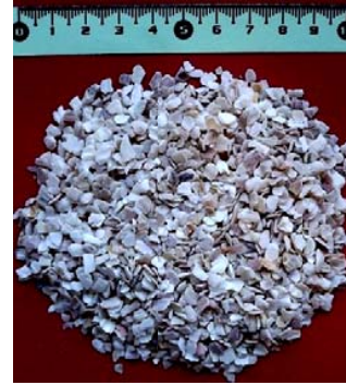
Fig. 2 Crushed Queen Scallop 2/4mm
