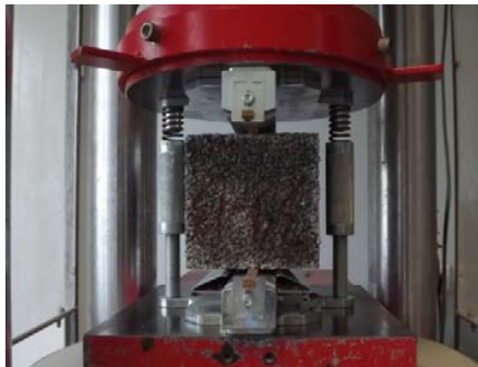
Fig. 3 Splitting tensile test
