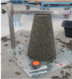
Fig. 5 Consistency of fresh concrete
