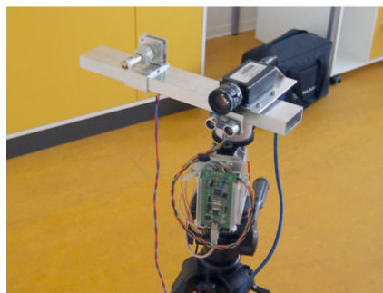
Fig. 1 The laser optical rangefinder
