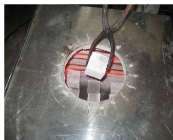
Fig. 2: Heating of sample in muffle furnace
