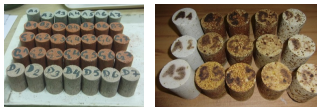
Fig. 3 Specimens before and after firing, fire 1, 2, 3
