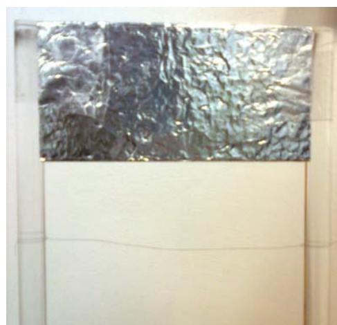
Fig. 1 A detail of the asymmetrical capacitor
