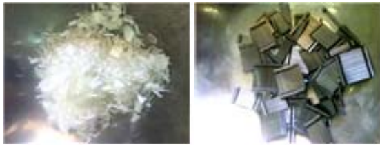
(a) PVA fiber (b) Steel fiber
