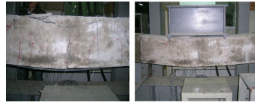
Fig. 13 Bonded FRP failure mode
