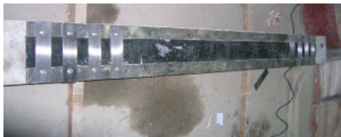
Fig. 7 Intermediate laminate FRP-strengthened RC structure
