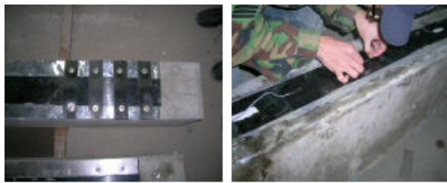
Fig. 6 Intermediate laminates and LVDT setup
