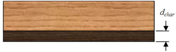
Fig. 2 Charring of timber – one dimensional
