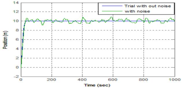
Fig. 12 Position simulation results with/without noise of PID
