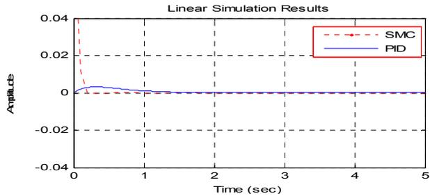
Fig. 7 Comparison for both controllers of cart's angle
