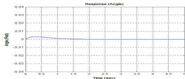
Fig. 3 Response for Pendulum's angle of PID
