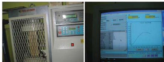
Fig. 2 The image of the pressing machine and the computer program used in the experiments
