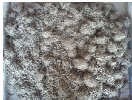
Fig. 4 Fiber ball Phenomenon (S44F1.25, S44V1.5, S51V1.5)
