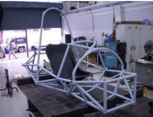
Fig. 14 Rapidamente92 student formula frame
