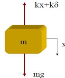
Fig. 2 Free body diagram of a mass-spring system
