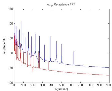
Fig. 13 The measured receptance for 80% cracked beam
