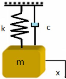
Fig. 3 Mass, spring and damper as a system
