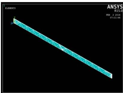
Fig. 10 Finite element modeling of the 20% cracked beam
