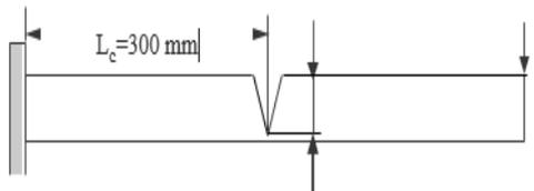
Fig. 8 Single cracked in 80% of width
