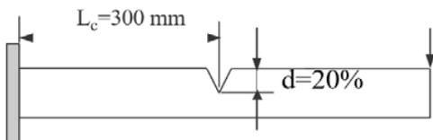
Fig. 7 Single cracked in 20% of width
