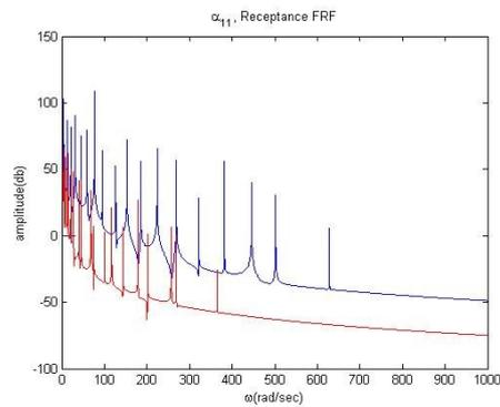
Fig. 12 The measured receptance for 20% cracked beam
