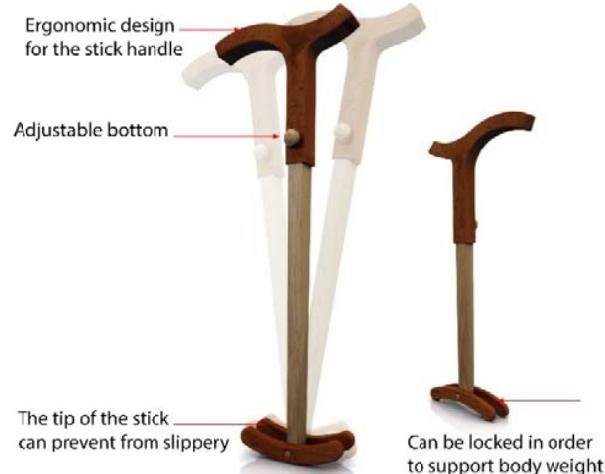
Fig. 4 Computer graphic model of the walking stick for the Elderly
