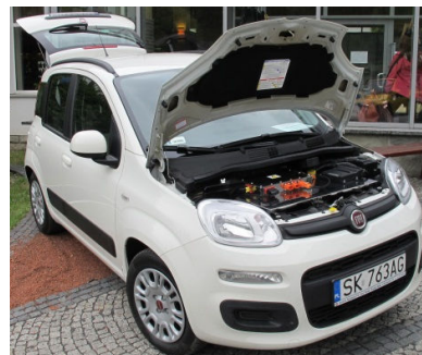
Fig. 9 Fiat Panda with Komel's traction motor – research and development project no. NR01-0084-10
