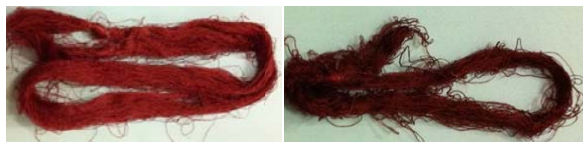
Fig. 4 Dyed silk yarn with Caesalpinia sappan Linn. and pre-mordanted using (a) 1% and (b) 5% alum solution. The darker shade was obtained from higher mordant concentration.
