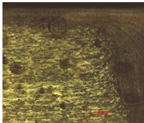
Fig. 7 (c) Microstructure of the THAZ zone in FSW weld
