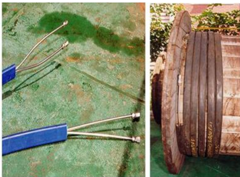
Fig. 4 Double Encapsulated Line and Coil of Control Lines
