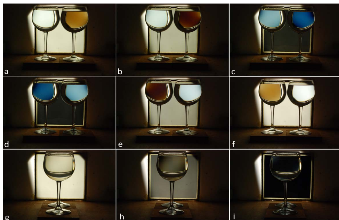
Fig. 9 (a)-(f) Rotation of polarization of fructose (on the left) and sucrose (on the right). When the polaroid in front of the camera is rotate, we can see sequences of colours in the two solutions which are one the opposite of the other. (g)-(i) Erase effect of the two laevorotatory and dextrorotatory substances
