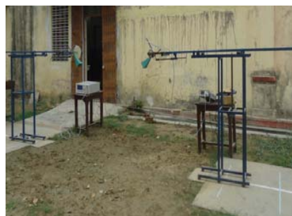
Fig. 1 Photograph of bistatic scatterometer system at measurement site
