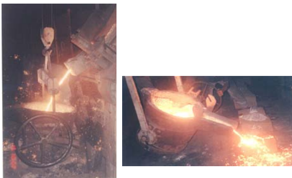
Figure 4 (a) Tapping and (b) Pouring of the molten metal.
