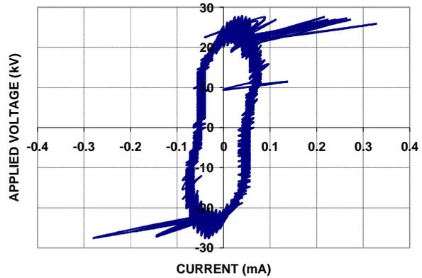
Fig. 7. Typical waveform of high RH lightly polluted specimen
