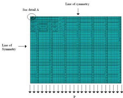
Fig. 3 1/4 FE model of integrally stiffened panel
