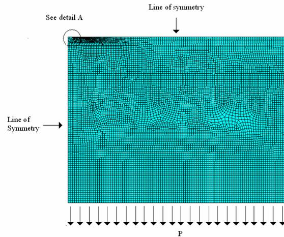
Fig. 4 1/4 FE model of unstiffened panel
