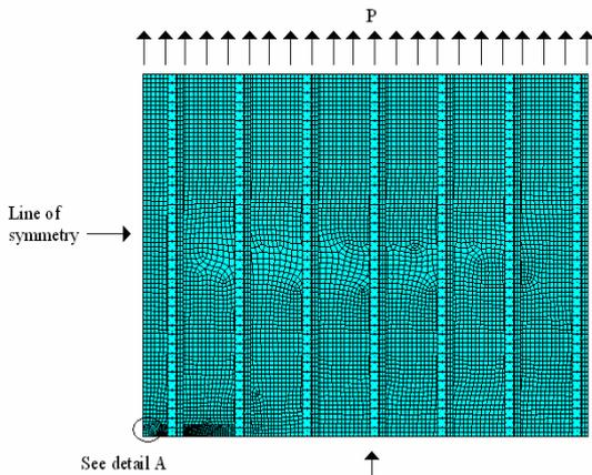
Fig. 2 1/4 FE model of riveted stiffened panel
