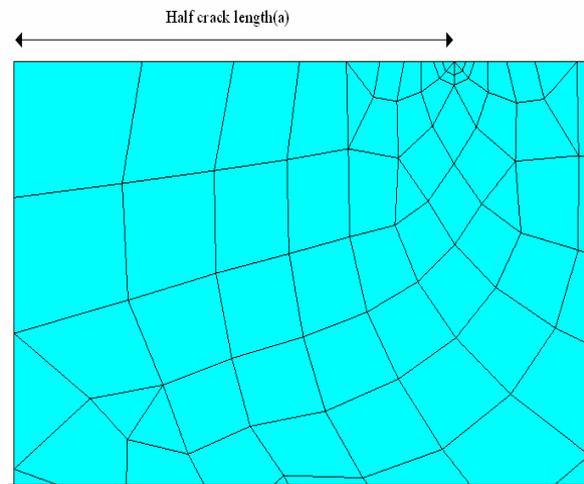
Mesh near crack tip
